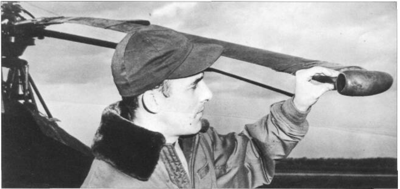
Above: An American airman examines the tiny rotor-tip jets which Friedrich von Doblhoff proposed to use to eliminate the effects of engine torque in his WNF 342.
